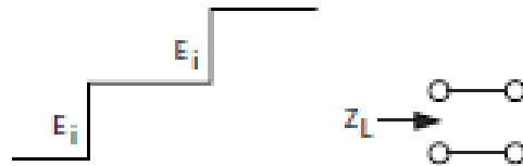
(A) Open Circuit Termination ( Z_L = \infty )
